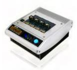
By combining the latest 64-bit architecture with the new 16 GB memory module, the Flashstream 2800F-MK2 currently supports device data files up to 125.5 Gb with theoretical device size support up to 8 Eb. Programmers that still utilize 32-bit architectures are limited to device data file sizes of less than 4 GB. As device densities and file sizes continue to increase, the 2800F-MK2 can handle the most demanding flash memory programming requirements.
