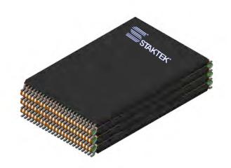
Stacking dimensions\*: L x W = 20.3mm x 12.9mm MAX 2-High = 2.34mm MAX Height 3-High= 3.48mm MAX Height 4-High= 4.62mm MAX Height
