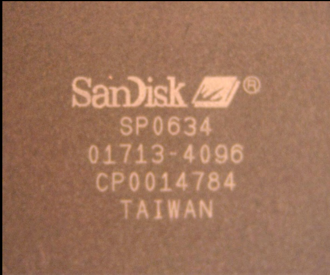
Device markings on flash chip contained within the Sony MemoryStick Duo memory card
