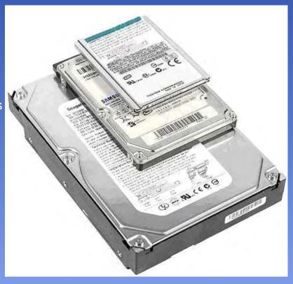
The reuse of Hard Drive Form Factors allowed for adoption of SSD technology quickly. This integration has grown as capacity and performance has closed the gap with mechanical drives.
