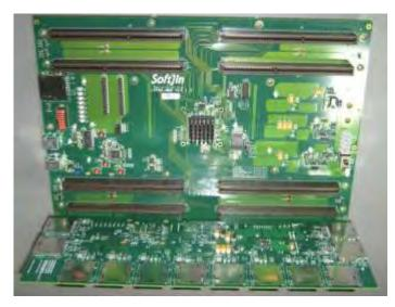
Picture shows one Image Processing and storage modules consisting of one memory base board and one memory board (having multiple SD Cards)
