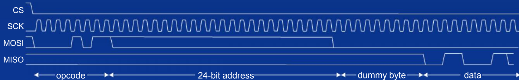
Fast Read command (opcode 0x0B), SPI mode, first byte read = 0x31
