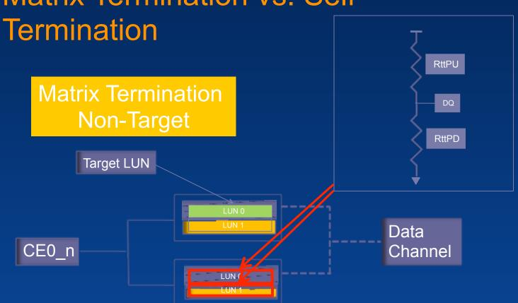
Multiple LUNs can be terminators providing a flexible array of termination values and locations
