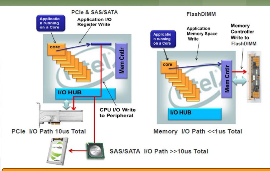
Memory Controller Path provides > 10X lower latency and 2X higher bandwidth
