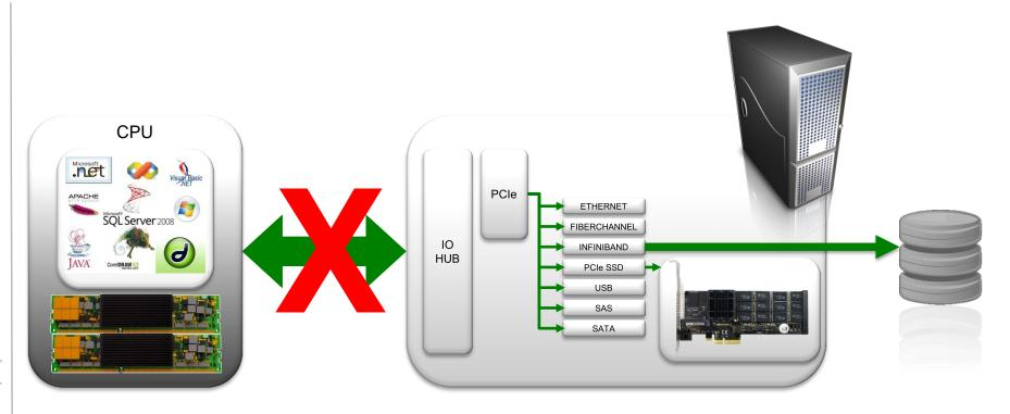
Connecting Flash to the Memory Bus eliminates arbitration and data contention on the I/O hub
