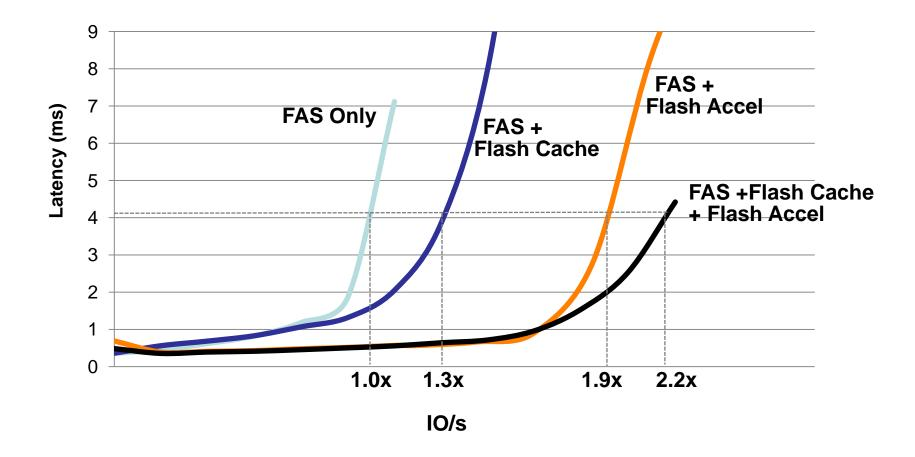
Note: Tested FAS3270 with SATA Drives, Micron P320 PCI-e card on ESX host
