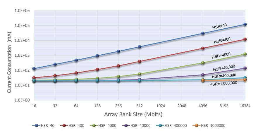
Large HSR enables low power and high density products, significantly reducing the sneak path and power consumption
