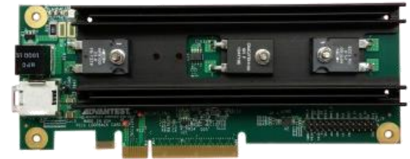
Test DUT with resistor and thermal sensor
