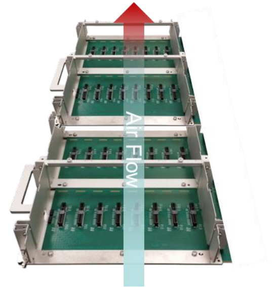
2 trays each with 2 rows of 8 DUTs
