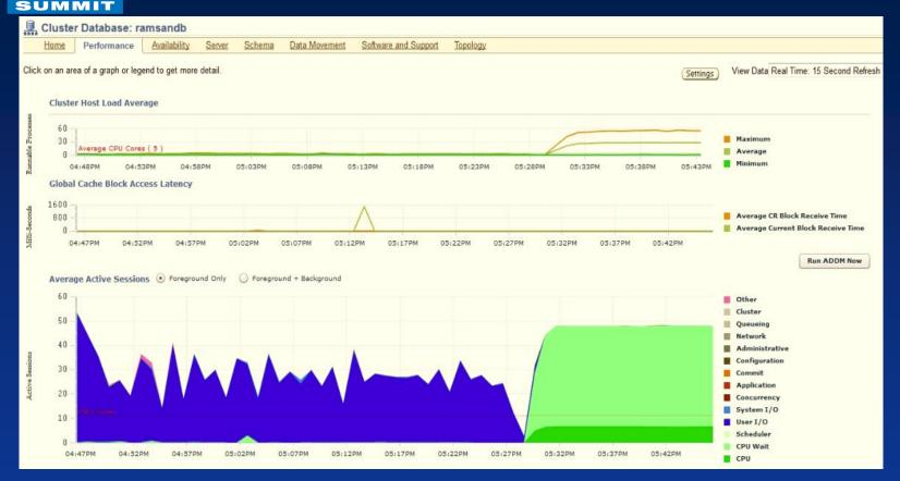
After switching to FlashSystem (05:27 PM), Disk IO wait disappears and waiting is now on host CPU. This graph shows the effect of the low latency of FlashSystem and how it increases host CPU utilization.
