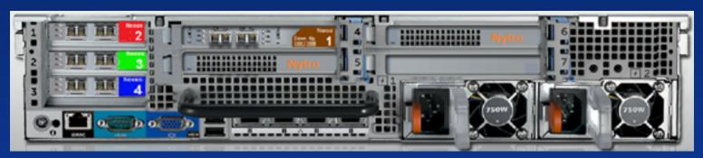
DCS-4000 with: 512GB DRAM, 8 8Gbps FC Ports, 4xGbe Ethernet Ports, 2x3.2TB LSI Nytro WarpDrive. Up to 3GB/s and 2M IOPS.
