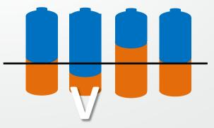
Separated storages, whole system fails when bad block count exceeds threshold in any disk Global storage pool, whole system fails when average bad block count exceeds threshold
