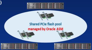
The solution enables shared server-side flash storage for Oracle RAC. This is the first configuration validated by Oracle using PCIe Flash.
