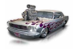
a device that increases the pressure of the fuel-air mixture in an internal combustion engine, used in order to achieve greater efficiency.
