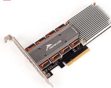
Memblaze flash validation platform with software NAND controller (only 1 channel valid)
