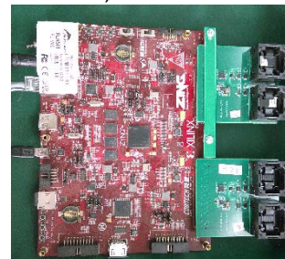
Memblaze flash validation platform with software NAND controller (only 1 channel valid)
