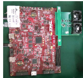
Memblaze flash validation platform with software NAND controller (only 1 channel valid)
