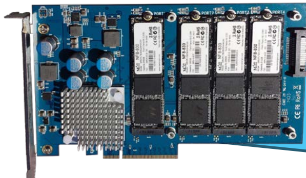
1 PCIe Switch Module = 4TB has 4 M.2 NVMe as Cache
