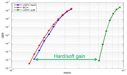
Soft-decision LDPC decoding has significantly better error correction than BCH decoding
