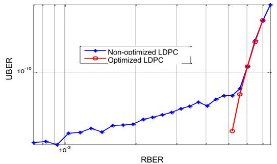
LDPC code parameters and decoding algorithm need to be optimized for good performance at low error rates
