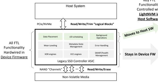
Key FTL Functionality Controlled with LightNVM in **Host Software**
