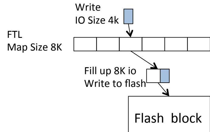
the system needs according to various scenarios IO model, unified consider defining each block size. **Match io model and Reduce write IO amplification.**
