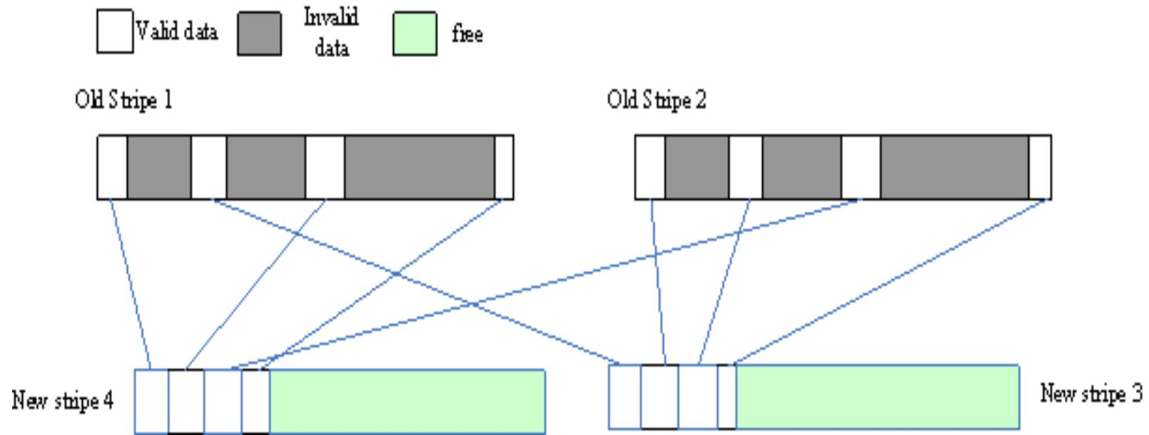
Based on the data validity, reclaim and reconstruct stripe, reduce rebuild stripe numbers (old stripe can free directly)
