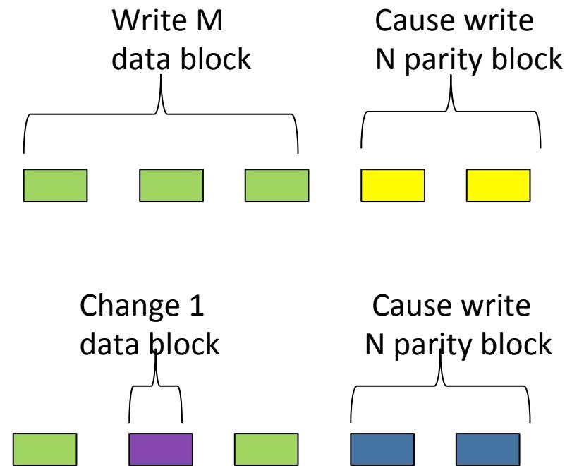
by garbage collection ,New write data always write new RAID stripe reduce parity block writing amplifier.
