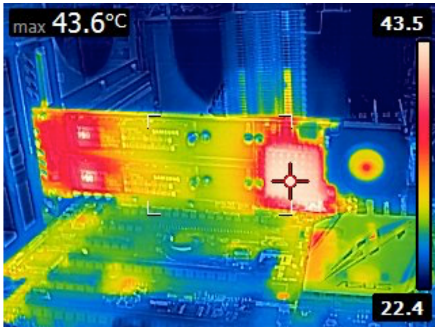
IDLE: M.2 drives at 45C, SLED at 45C
