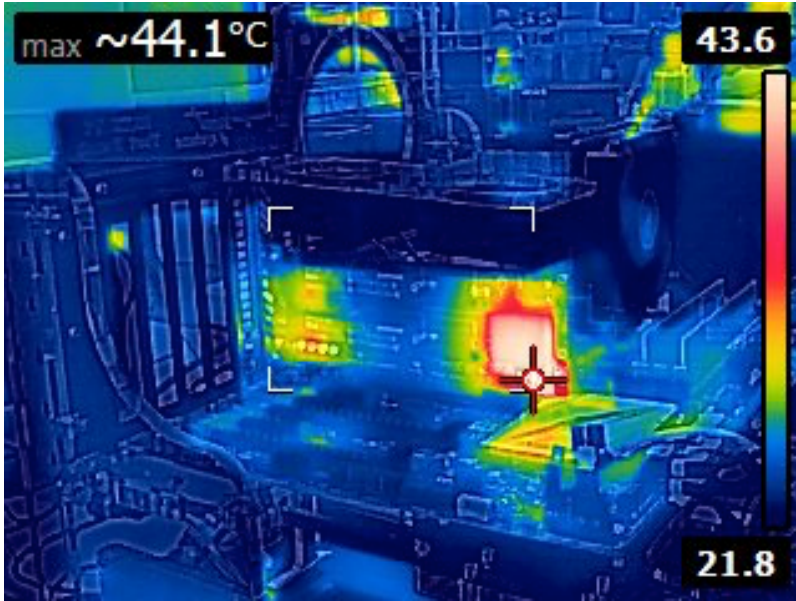
IDLE: M.2 drives at 35C, SLED at 45C
