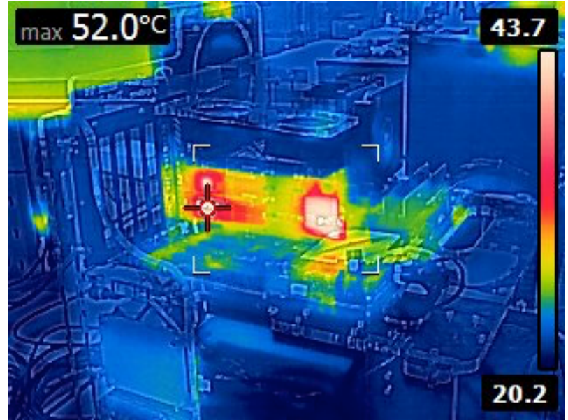
LOAD: M.2 drives at 50C, SLED at 45C
