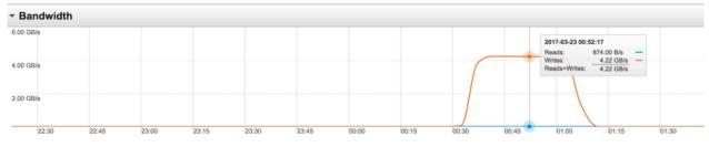
Test Started 0:33:12 and finished at 1:12:16 = 39 minutes - Running at 4.2GB/s Write Average
