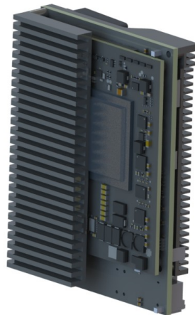
RAID Controller side
