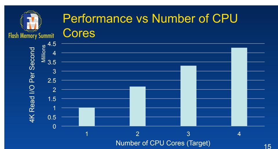
System Configuration: 2x Intel® Xeon® Platinum 8180 CPU @ 2.50 GHz, Intel® Speed Step enabled, Intel® Turbo Boost Technology enabled, 4x 2GB DDR4 2666 MT/s, 1 DIMM per channel, Ubuntu\* Linux 17.10, Linux kernel 4.13.0, SPDK 18.04, DPDK 18.01, Mellanox® ConnectX-4 MT27700
