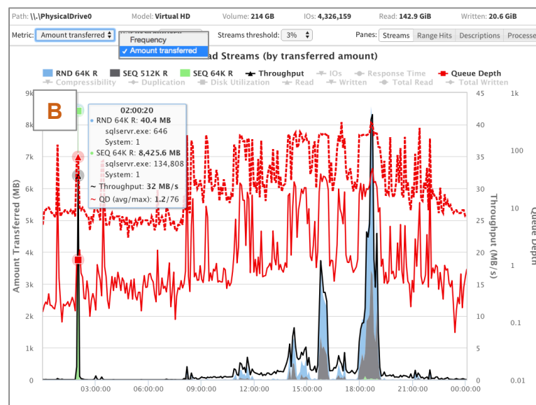
B IO Stream Map by Amount Transferred – Throughput in MB/s MB/s, Ave/Max Queue Depth
