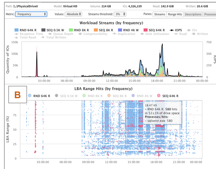
B LBA Hit Range – by Frequency (IOPS) IO Hits selected by IO Rate (Frequency)
