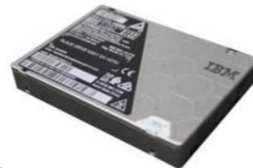
IBM FlashCore Module Ref: B. Yardley, "Spin Torque MRAM Is Ready for Applications Today", MRAM Developer day, August 2018
