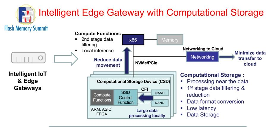
CSD at the Edge performs 1<sup>st</sup> stage data processing, filtering and reduction, before transferring data to DC and/or Cloud
