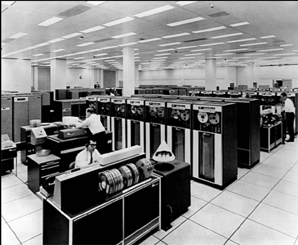
IBM Mainframe room with Core Mem and Tapes as Input + cards/Output with Printer and to Tape
