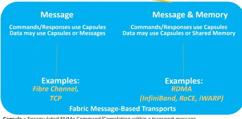
**Capsule** = Encapsulated NVMe Command/Completion within a transport message **Data** = Transport data exchange mechanism (if any)
