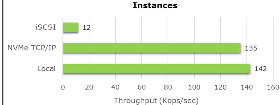
Minimal Performance overhead with NVMe over TCP/IP
