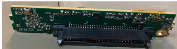
NVMe-oF Converter Controller Interposer (SSD side)
