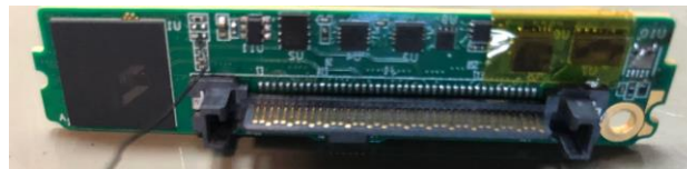
NVMe-oF Converter Controller Interposer (network side) (*8639 is used to drive 2x25Gb Ethernet)
