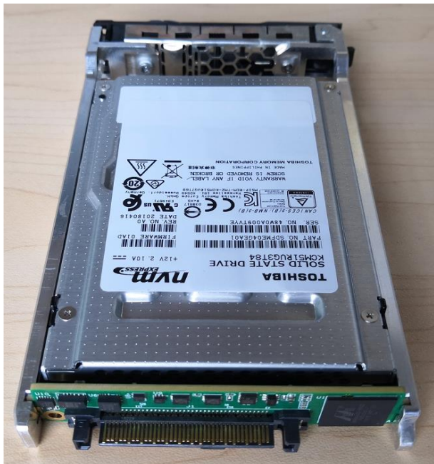
NVMe-oF Converter Controller interposer in a carrier
