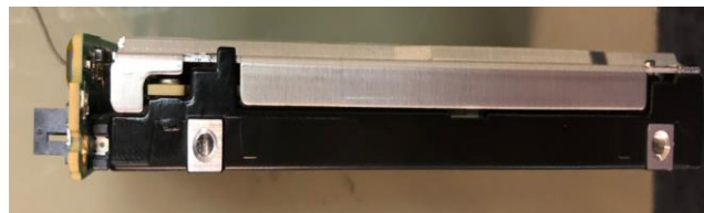
NVMe-oF Converter Controller Interposer (profile) Connected to U.2 (non-carrier)
